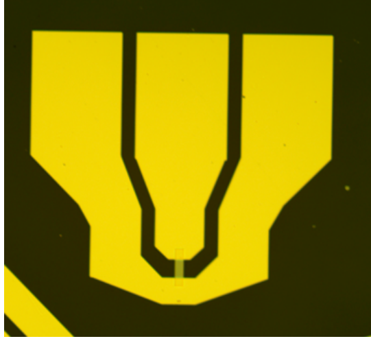
Figure 3.5.: Microscopic image of a device to perform the ST-FMR measurement. The large area in gold represents the gold contact pads for the RF probes. The small bar attached to the two pads is the material being probed.
