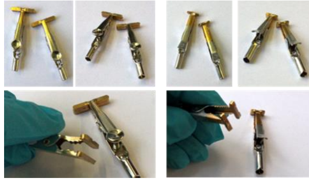
Figure 7.1: Metal clamps developed in two sizes to measure the electrical properties of unstrained conducting samples.
