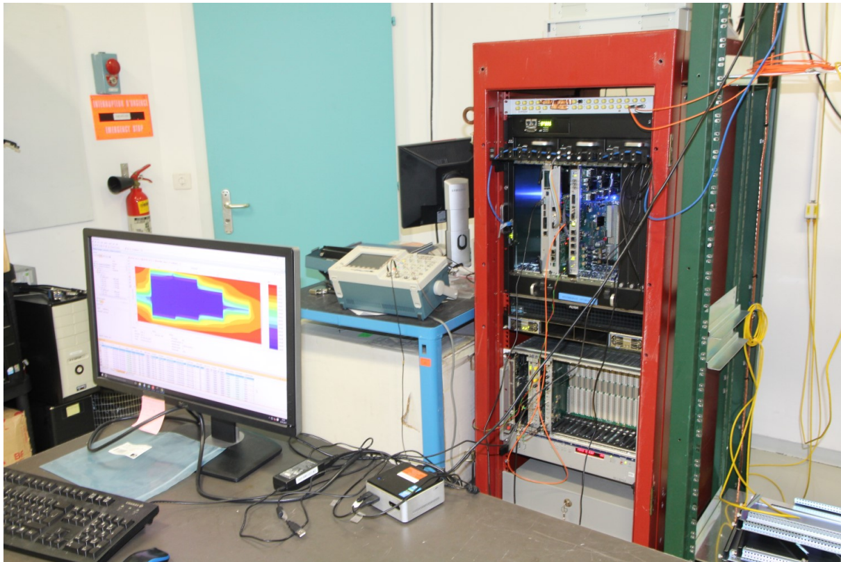
FIGURE 9.16: Setup used for the integrated tests with the FTM. Both boards were inserted in the upper level of the red rack with up to two FOX prototypes on top of it as the entire fibre handling was done via the backplane.
