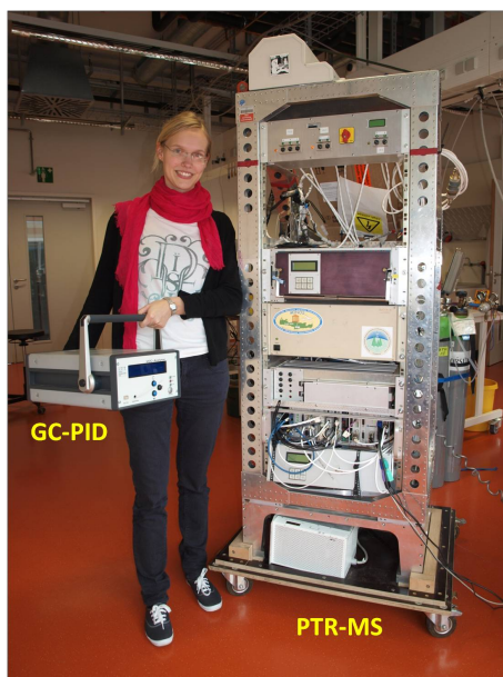
Fig. 2.6: Two detectors for CRM total OH reactivity measurements: To the right the IONICON PTR-MS, to the left the GC-PID.
