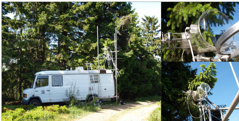
Fig. 4.1: Cuvette set-up in the field on Kleiner Feldberg, Taunus, Germany: The enclosure system was fixed at a Norway spruce branch. The instruments (Sensors, PTR-MS, CRM) were located in the van underneath to keep inlet lines short. For 17 minutes the lid was kept open to allow contact with the natural atmospheric environment and closed automatically for 3 minutes.
