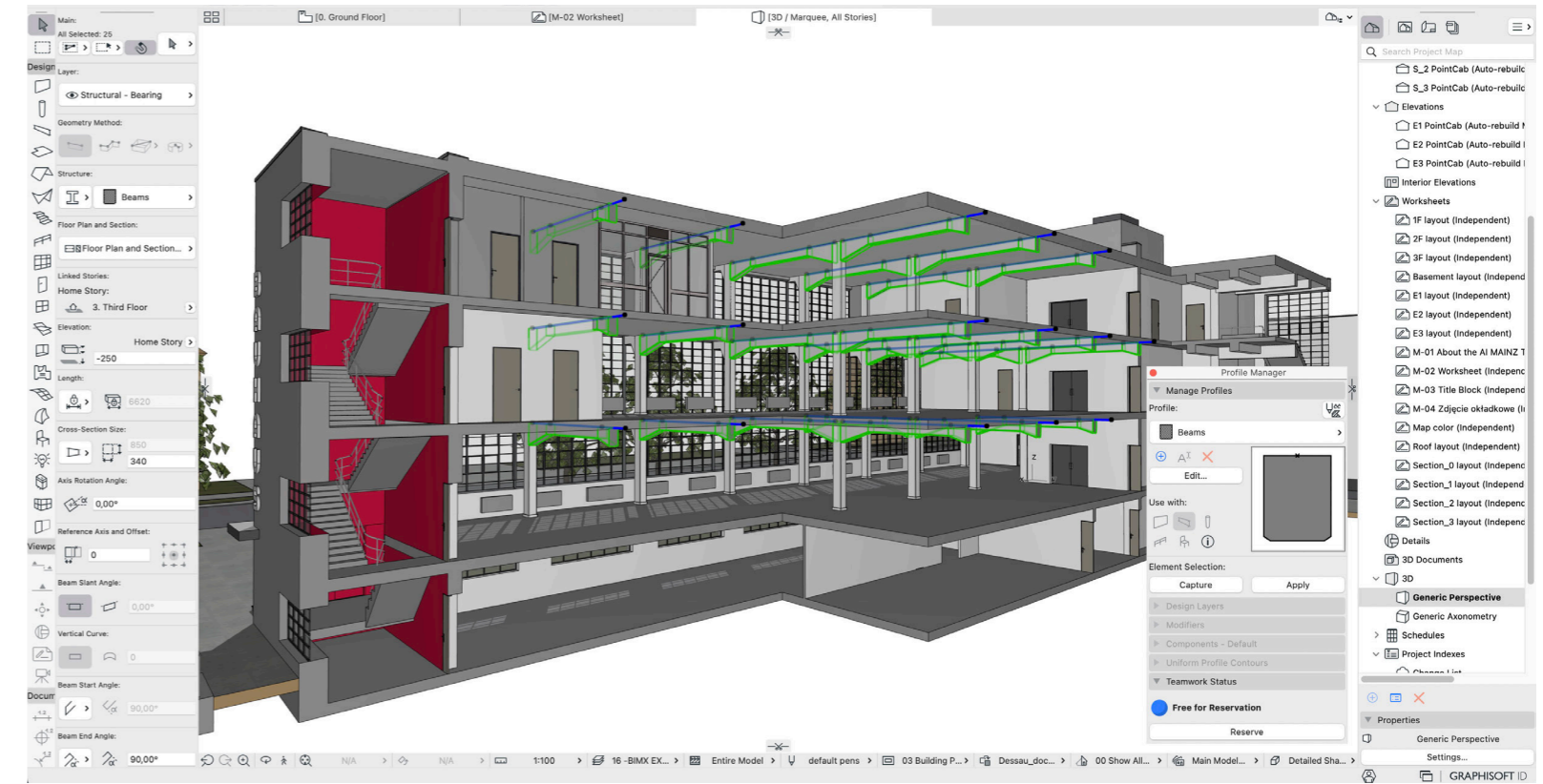
Fig 5. Different profiles were created to maintain the original and real building monolithic structure (AI MAINZ/Karol Argasiński, 2023).
