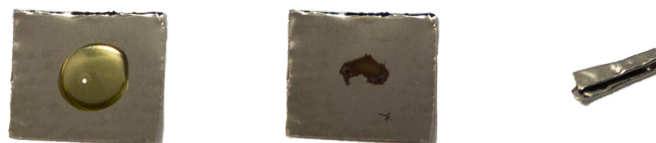
Figure 4.18: Photographs of the sample preparation process. From Left: Drop of acid solution containing the natural Pd on a 5 \times 5 \text{ mm}^2 metallic Zr foil. Center: Sample after evaporation of the solution. The residue of the solution is visible as dark spot. Right: Folded sample, length 2.5 mm. See text for further description.
