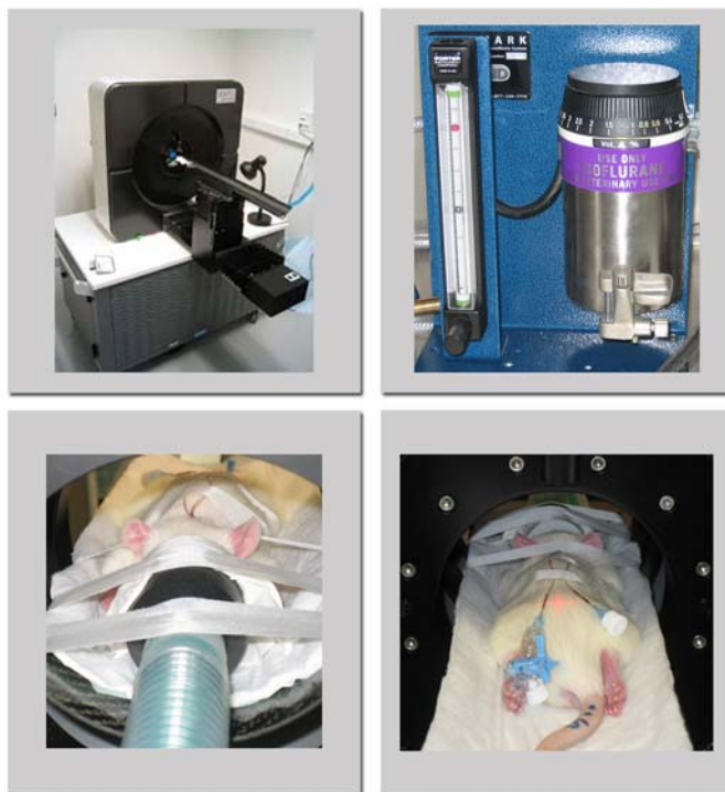
Figure 12: Positron emission tomography equipment. PET camera was a Siemens/Concord Microsystems Focus 120. Anesthetic was isoflurane at a concentration of 1.8 %. Animals were anesthetised and catheterised. The head was tape-fixed to minimize image blurring trough head motion.
