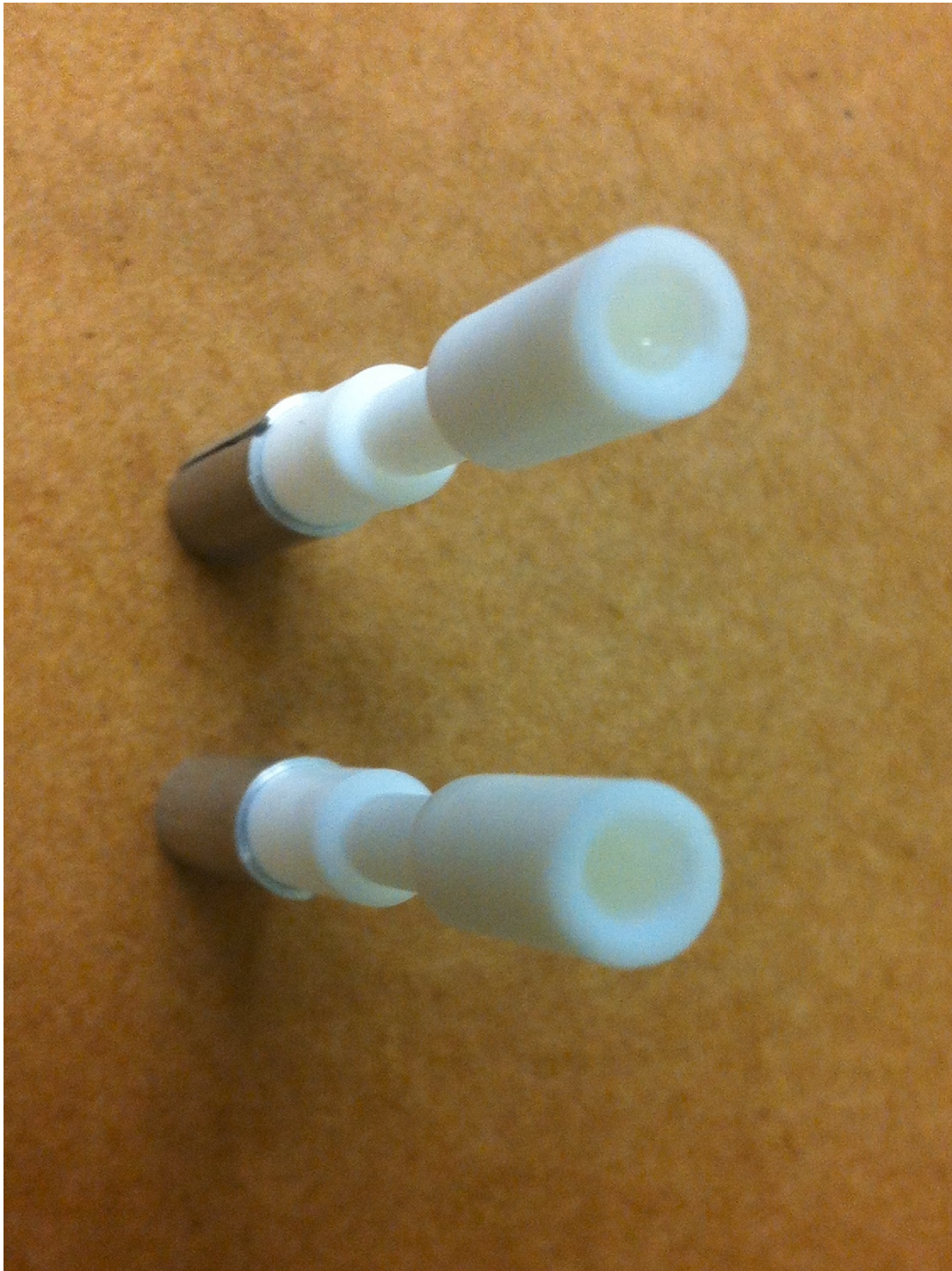
Fig. 16. Two sample holders shown with their sample cavities filled with petroleum jelly (slight yellow tint). Aluminum sleeves that protect the sample holder during winding of the serial inductor coil are also depicted here.
