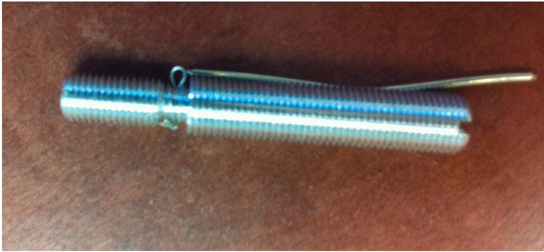
Fig. 20. Soldering the connection loop into the inner conductor is performed with an ultrasonic soldering iron.
