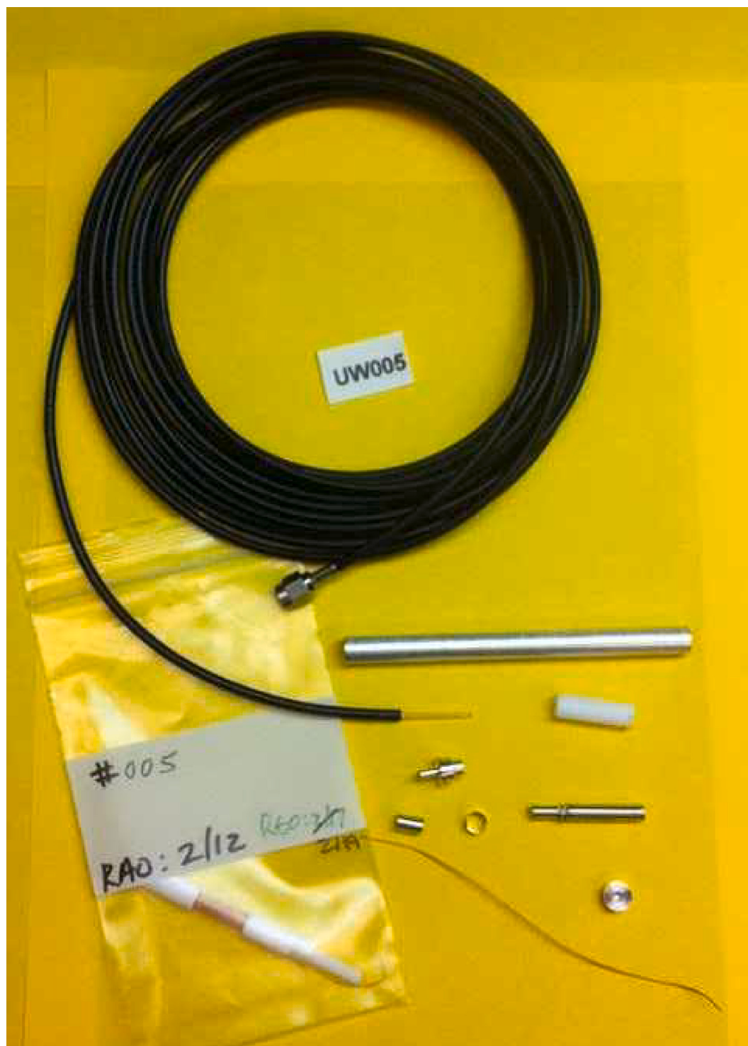
Fig. 14. A typical assembly kit for a single NMR probe containing all required construction pieces. For quality control purposes, the individual assembler of the probe are indicated on the bag and each probe was assigned a unique identification number.
