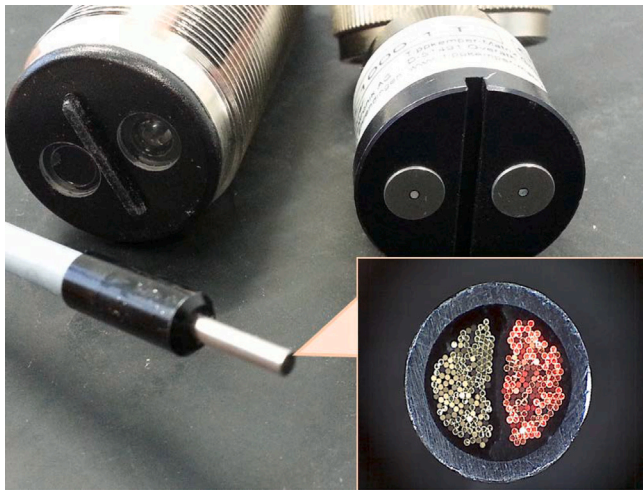
Fig. 3. Photographs of the Tippkemper-Matrix IRS-U2LA optical sensor and the bisected light guide. The upper left part shows the head with the infrared emitter and the optical sensor. The two ends of the light guide are shown in the lower left and upper right parts. An enlarged view of the two combined sections of the fiber bundle is shown in the insert. For this photograph the two sections were illuminated differently. In the upper right part the adapter with the divided sections is shown.
