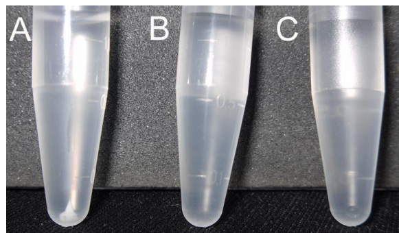
Figure S7. Optical image of reaction products A) in the presence of silicatein- \alpha , B) using only buffer (TBS, pH 7.4) and C) using denatured silicatein- \alpha . Formation of a white precipitate ( \text{SnO}_2 ) is only visible in the presence of functional silicatein (A).
