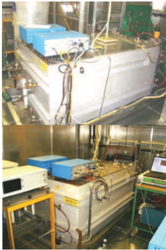
Figure 6.1: The ASTEC power supplies located in the ISOLDE's HV cage.
