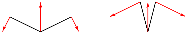
Figure 9.20: In the case of the first model of a cable, the curvature forces where orthogonal to the segments: there is no interference between the curvature and length forces.
