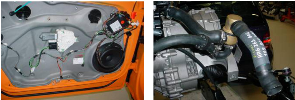
Figure 1.1: Some of the one dimensional parts encountered in a car: on the left some cables in a door, on the right a hose
