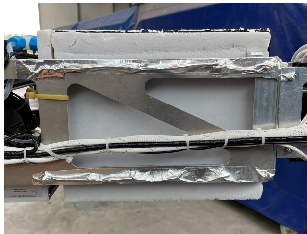
Figure 2. Ozone instrument with insulation as mounted inside the TPC-TOSS in the rear part.
