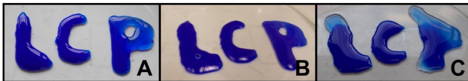
Figure 8.7. After annealing Co-LCP (A) for 2 d at 130 °C, a gel has formed covered by a “skin” (B). Exposing (B) to humidity for 1 d results in (C) which appears liquid-like again.
