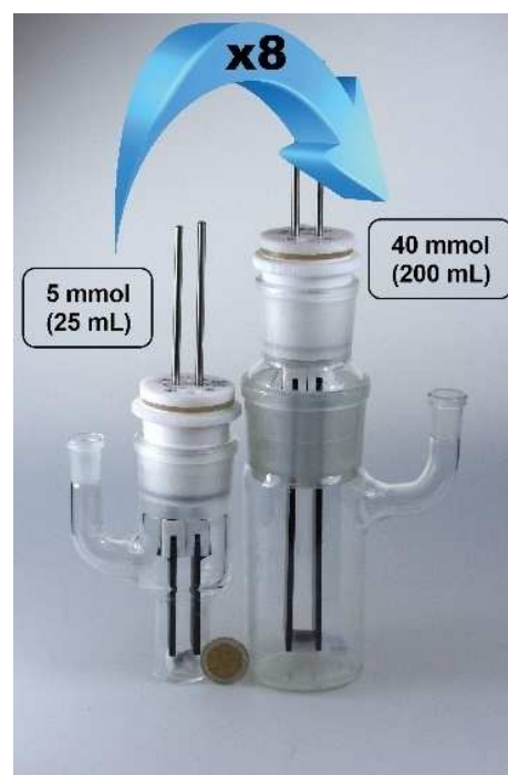
Figure 2. Scale-up from a 5 mmol to a 40 mmol batch. For size comparison of the beaker-type cells a 2 € coin is placed in front (diameter 25.75 mm \approx 1.01 in).
