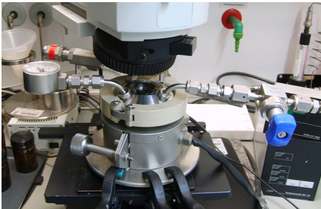
Figure 10-4. Gas phase reactor after installation and during olefin polymerization
