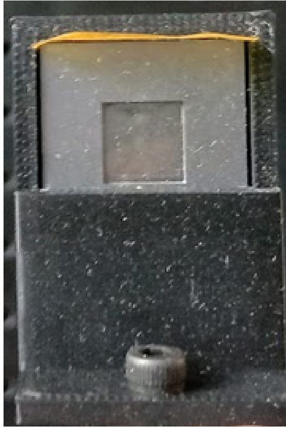
Figure 7.3: Photograph of the diamond plate, mounted in a 3D printed support structure for measurements in the interferometer.
