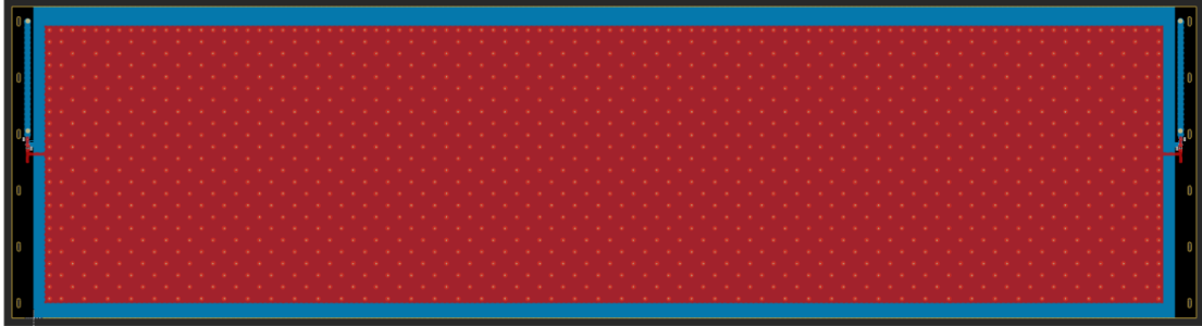
Figure 4.46: CAD drawing of the Starry Night cathode, oriented with the top towards the spectrometer magnets, with blue showing the exposed copper on active area side and red that on the other. Visible in this red area as white dots is the hole pattern, with each hole having an LED positioned above it. Image from [88].
