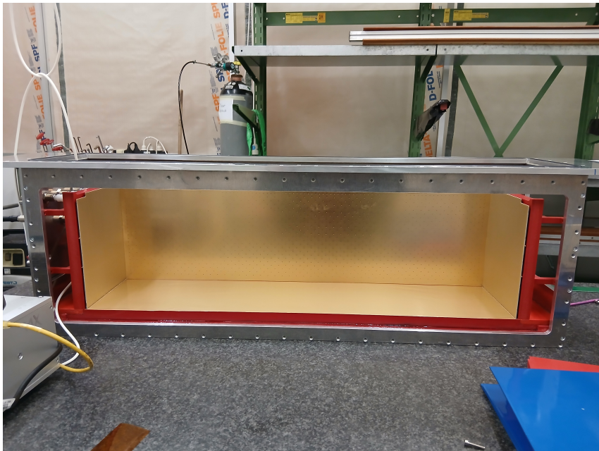
Figure 5.10: Interior view from the direction of amplification stage into the interior of the active area. The two field cage PCBs on the side are glued onto the red polyvinyl chloride blocks behind them. The large vertical plate in the middle is the cathode, with the holes for Starry Night visible, though the Starry Night modules themselves are not yet installed. The horizontal surface is the exit foil, stretched and glued into the polyvinyl chloride frame.
