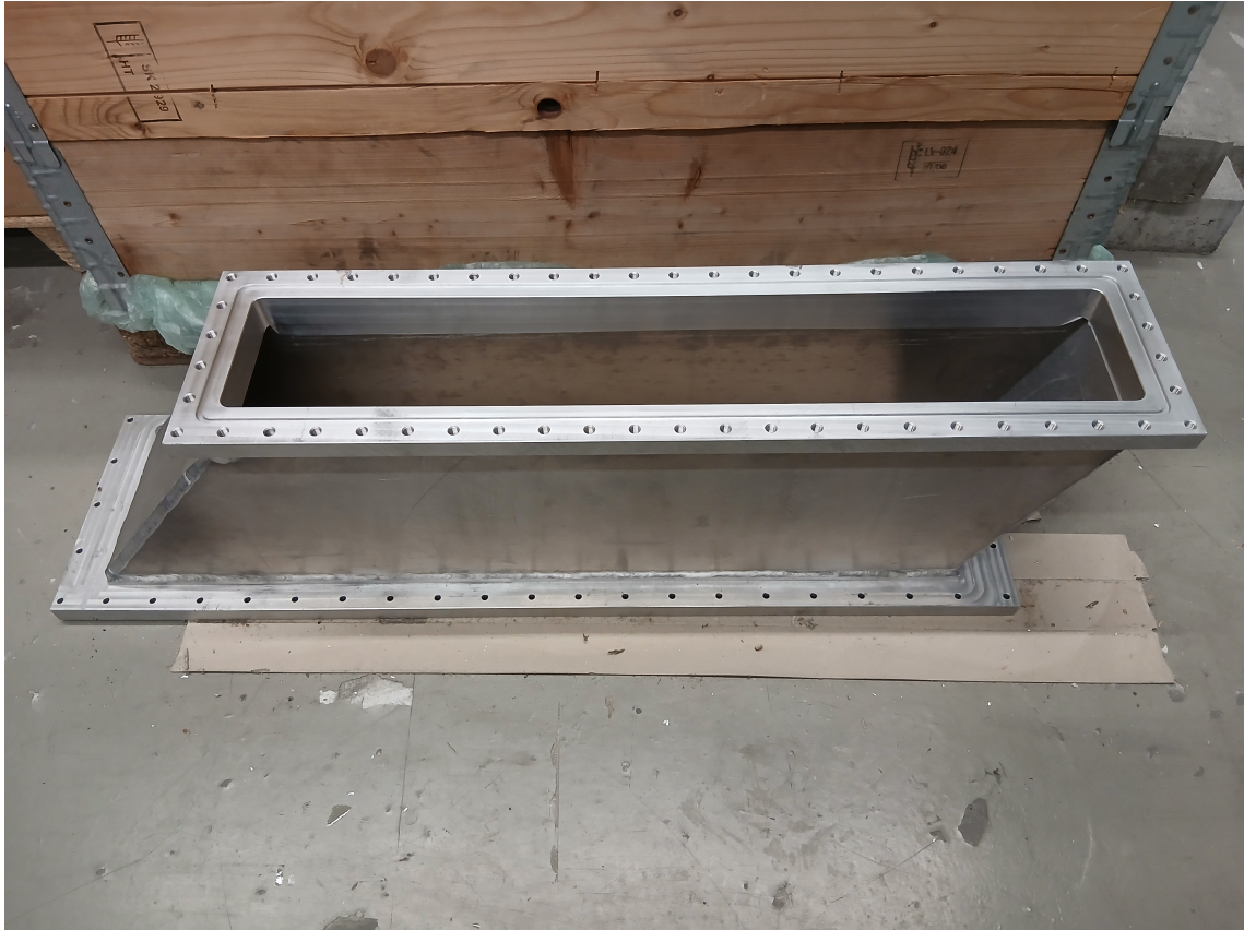
Figure 4.8: Spectrometer connection frame, assembled out of six parts that were welded together.
