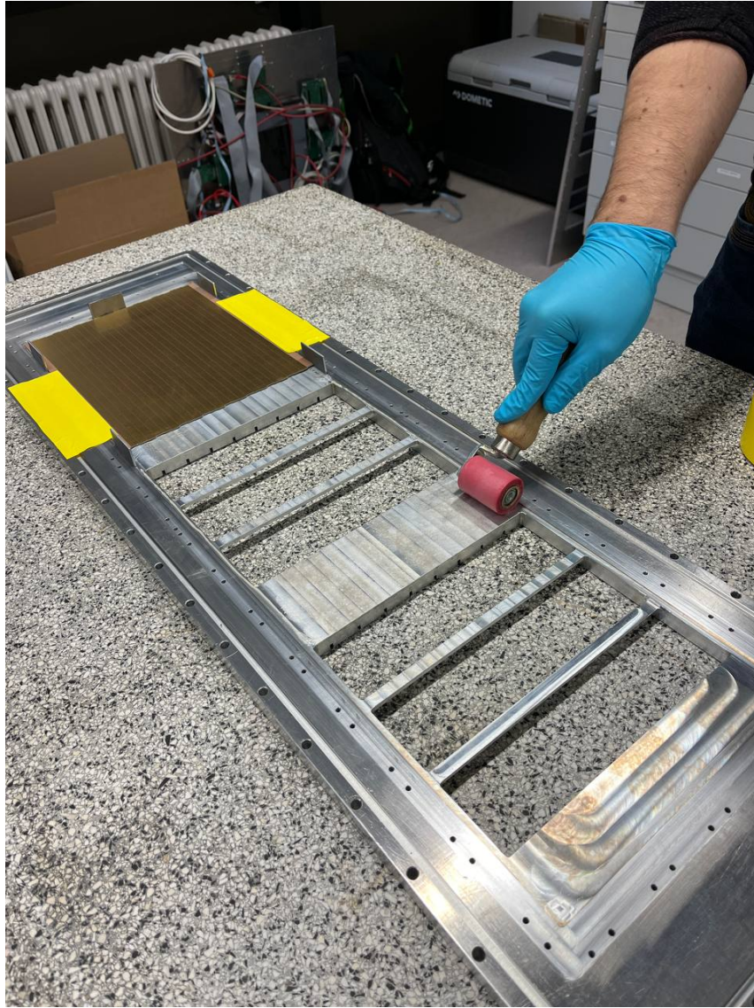
Figure 4.17: A single readout PCB glued into their aluminium frame, with the glue being applied for the next one. The yellow tape fixes the PCB in place.
