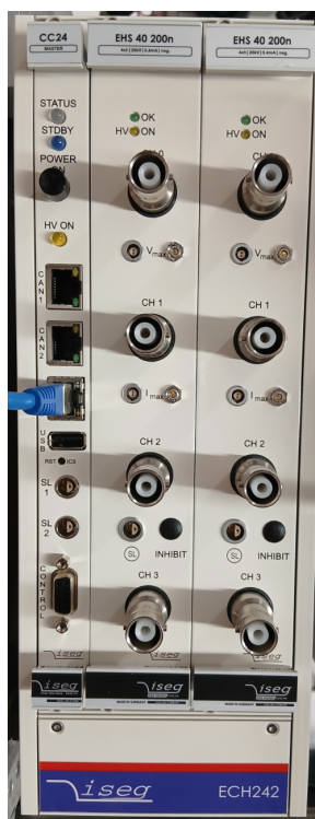
Figure 4.12: 2 EHS 40 200n voltage supply boards and CC24 control board mounted in an ECH 242 crate.
