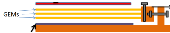
Figure 4.18: NS2 Stretching Systems, as developed by CERN for the new generation of CMS GEM foils. Image from [67].
