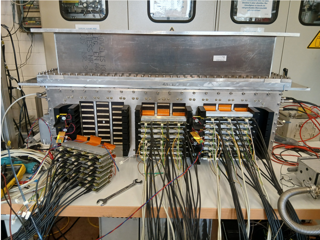
Figure 5.11: Front view of the completed TPC. The field cage extension it is connected to consists of only the frame, with no components installed. This is done to achieve gas tightness until the components of the extension can be installed. The yellow tape covering the NS2 screws from figure 5.1 has been removed, as those screws have been topped with glue.
