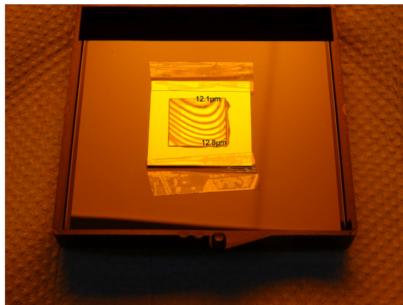
Figure 7.4: Diamond Plate measured in thin-film interference setup by the manufacturer Diamond Materials. The lines are an interference pattern generated by testing equipment of the manufacturer and show the surface topology with 130 nm thickness variation between each ridge. Variance between these points is unknown and as such this measurement itself is insufficient to reach our desired degree of precision.
