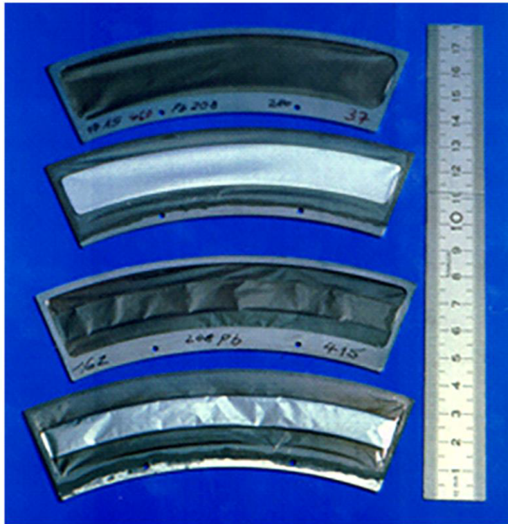
Figure 1.5.: ^{208}\text{Pb} -targets showing the backing side (1 and 3 from above) and the target side (2 and 4 from above), respectively, with an enlarged target area and improved backing quality (upper two) compared to the previous target version (lower two). From ref. [120] The targets illustrated show the development of target segments for the target wheel for SHIP experiment setup at the GSI Darmstadt. It shows the improvements on the way to the perfect PbS target.
