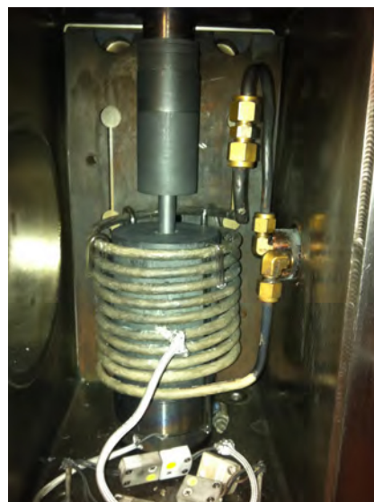
Figure 2.1: Schematic of induction hot press setup (left) and picture of hot press taken at Caltech (right).[107] The powdered sample is loaded into the die and covered with grafoil on all sides. Pressure is attained with a graphite plunger and the induction coil is utilized to heat up the die.
