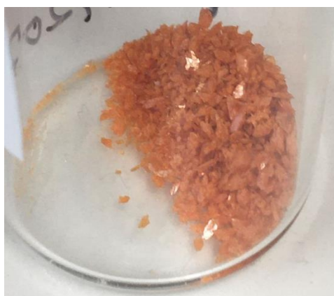
Figure S2. Photograph of crystals of [\text{Cr}(\text{dgpy})_2][\text{PF}_6]_3 \cdot 1.5 \text{ DMF} .
