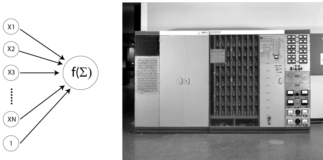
Figure 4.8: Sketch of the the working principle of the Perceptron (left): The inputs are agglomerated in a weighted sum and then handed of to an activation function f . On the right: the realization of the Perceptron as hardware network. The adjustable weights were realized by potentiometers stored in the center cabinet. Courtesy of the National Museum of American History.
