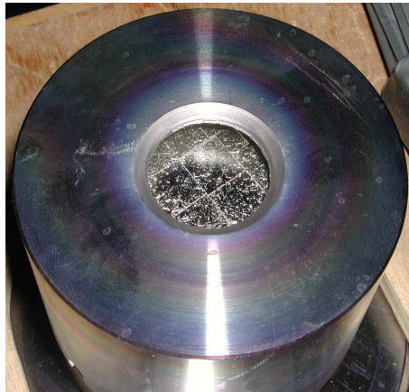
Figure 2.3: \text{Co}_2\text{FeSi} target mounted on a sputtering cathode.
