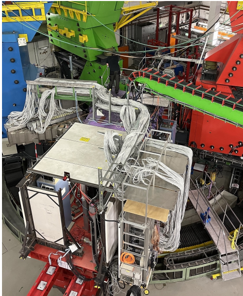
Figure 6.4.: KAOS installed within the A1 setup. It allows for detecting particles under 0^\circ forward angles and is best suited for observing kaons.
