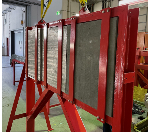
Figure 7.5.: Lead absorber plate from inside KAOS to suppress positrons.
