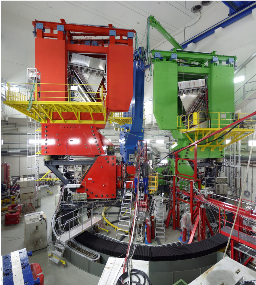
Figure 3.3.: The A1 experimental hall with the spectrometers A in red, B in blue and C in green. Spectrometers A and C are shown with opened shielding houses, revealing the detectors. The beam enters the hall through the thin beam pipe on the right.
