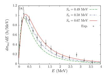
**Fig. 5** Sensitivity of breakup calculation to the <sup>18</sup>C-n binding energy for <sup>19</sup>C impinging on <sup>208</sup>Pb at 67*A* MeV. LO Halo-EFT <sup>18</sup>C-n potentials are fitted to reproduce three binding energies at the centre (0.58 MeV, blue dash-dotted line), lower bound (0.49 MeV, green dashed line) and
