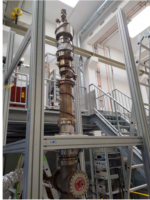
Figure 3.20.: The vacuum vessel of the electron cooler test bench during bake-out preparations.
