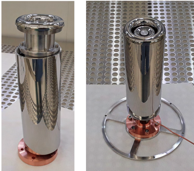
Figure A.14.: Pierce electrode in HIM cleanroom during source assembly.
