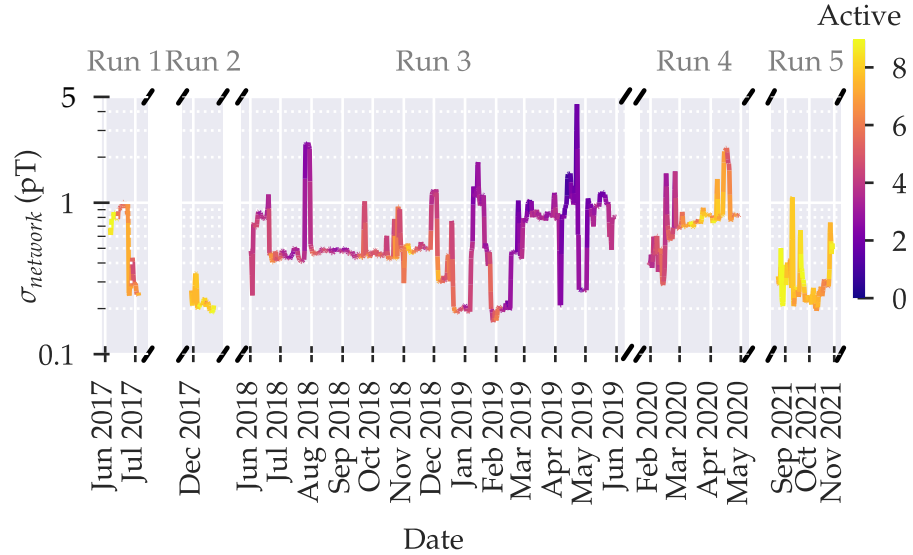
Figure 4.6: Overview of the sensitivity during the GNOME science runs. One-day rolling average of the standard deviation of the network. This is calculated according to Eq. (4.1). The standard deviation is calculated over a second of data. Then this information is averaged for one hour.
