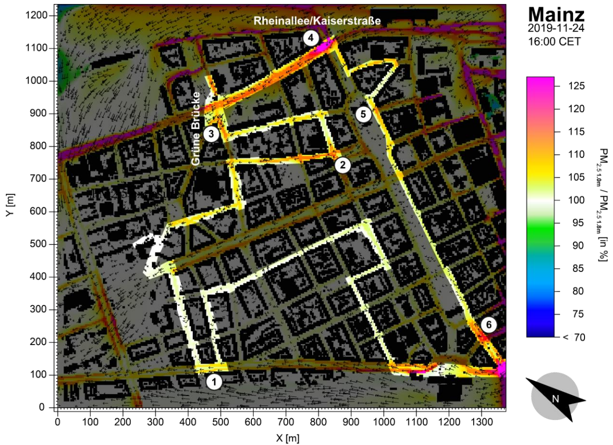
Fig. 2-7 Simulated relative differences distribution of PM 2.5 concentrations between 1.0 and 1.8 m in the study area with the measurement route highlighted. The colors display reduced (blue and green), equal (white) and increased (yellow to red/magenta) PM 2.5 exposure at 1.0 m level. The arrows represent horizontal wind speed and direction.
