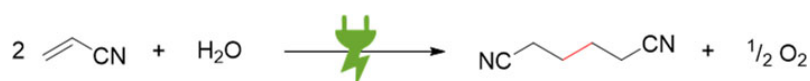
Scheme 1. Used technical electrochemical process called Baizer process: electro-conversion of acrylonitrile in industrial processes.
