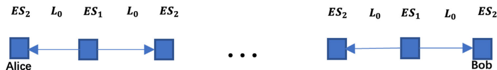
Figure 2. Schematic of the long-distance entanglement distribution protocol including two types of elementary stations: ES_1 to send the light mode and ES_2 to receive it.
