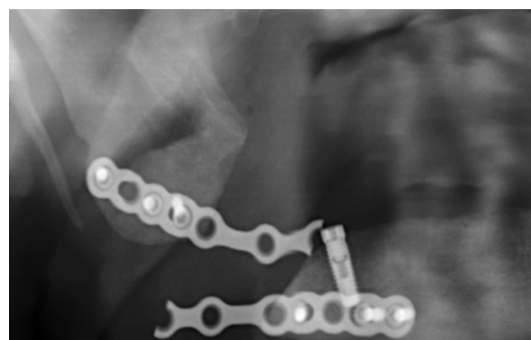
FIGURE 11 Panoramic X-ray of a fractured alloplastic reconstruction plate.
