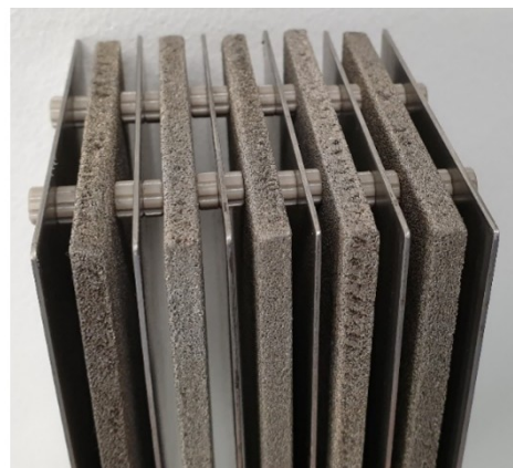
Figure 7. Bottom view of the electrode stack. The nickel foam sides are separated from the stainless-steel cathodes by screws made of polyether ether ketone (PEEK, thickness per side 3 mm). The anode geometric surface area in contact with the electrolyte is 1225 \text{ cm}^2 . The foams have a thickness of 5 mm. The stainless-steel sheets have a thickness of 1 mm.
