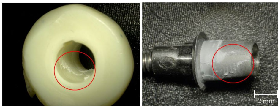
Fig. 7 Representative sample for mixed adhesive fractures. The red circles show the resin cement partially remaining on the titanium surface (right) with the corresponding area free of resin cement on the crown (left)
