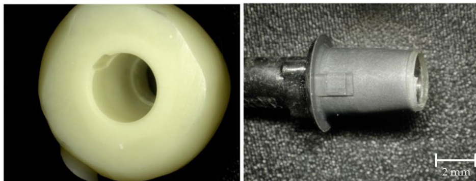
Fig. 6 Representative sample for complete adhesion of resin cement to titanium base
