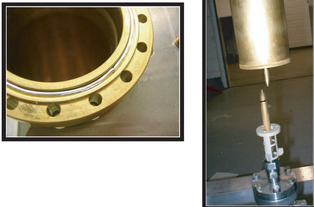
Figure 3.6: Left: indium sealing between the chamber body and the UMF (the inset was still not inside). Right: Pinch-off tube directly after performing the cut.
