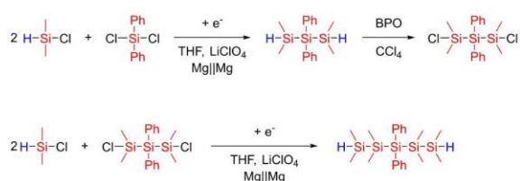
Scheme 7. Synthesis of oligosilanes via reductive coupling, followed by chlorination of hydrosilanes, BPO = benzoyl peroxide. [56,87]
