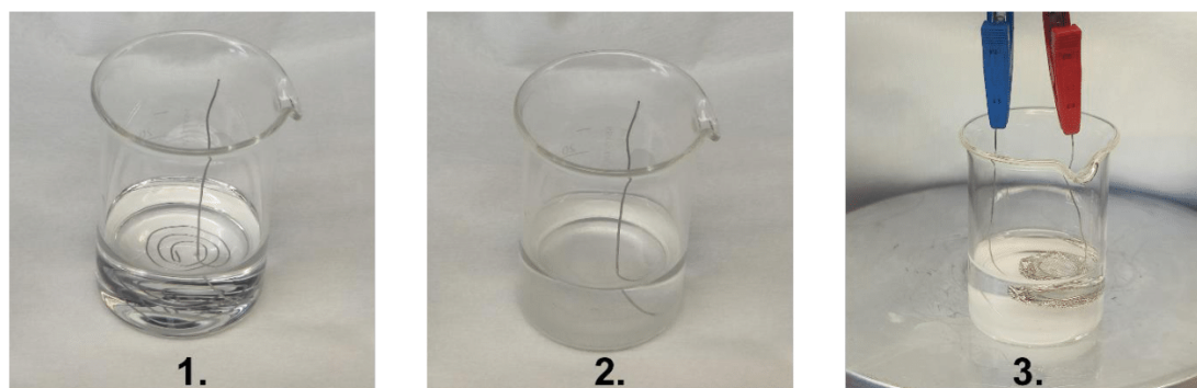
Figure 4. General procedure for optimization reactions in horizontal cell design: 1. the glass cell compartment was charged with the electrolyte and MeOH and the cathode was added; 2. the cathode was evenly covered with quartz sand; 3. the anode is connected to an alligator clip and after adjusting of the inter-electrode gap, the cathode is connected to an alligator clip.
