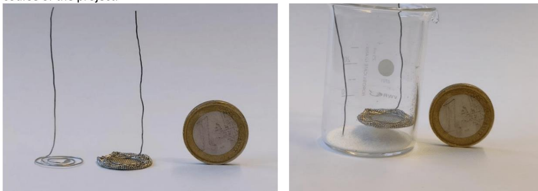
Figure 2: Horizontal cell design for the reduction of \text{SiO}_2 ; left: 20mm diameter platinum gauze anode, platinum wire (5.6 cm helically coiled, 0.4 mm in diameter), with 1 Euro coin for size comparison; right: setup with cathode covered in quartz sand, with 1 Euro coin for size comparison.
