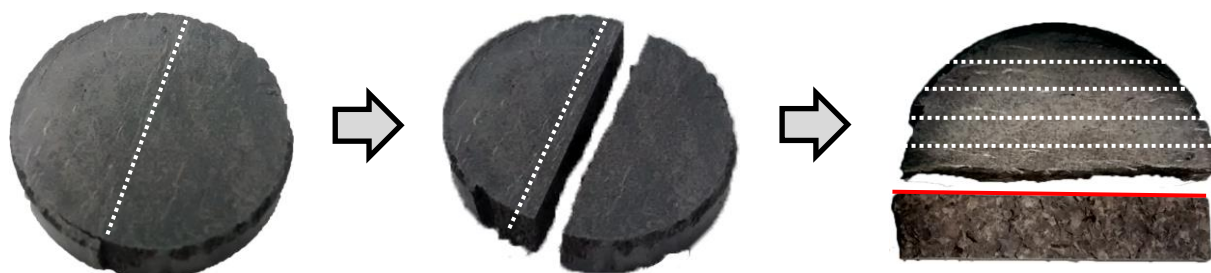
Figure 22: Preparation of diffusion profile samples for IP measurement from diffusion of 8 \times 10^{-6} M Np into OPA. The dotted line indicates the cleave locations, the red line the interface between the bore core and the Np solution of the primary reservoir.
