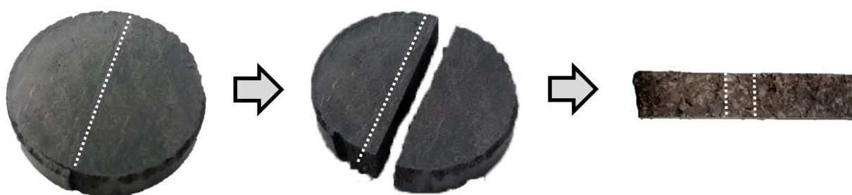
Figure 18: Preparation of the diffusion profile samples from OPA bore cores (diameter 2.54 cm, height in this case 5 mm). When possible, the bore cores were cleaved (dotted lines) along the bedding as it was eased.
