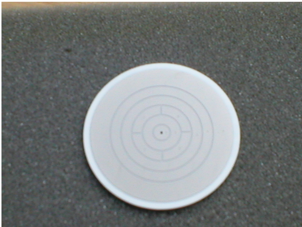
Figure 3.4: Real trap's front side. The light-gray surface is metal and the dark-gray lines and white border is isolating material.
