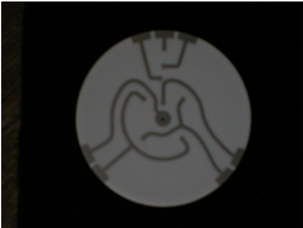
Figure 3.5: Real trap's rear side. The contact feedthroughs connect the electrodes on the front with the lines in the rear. The contact lines end up in the border of the trap, so as to clamp them to individual channels which go the exterior of the vacuum chamber.
