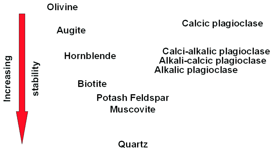
Figure 2.6: Goldich's sequence of mineral susceptibility to weathering. Minerals listed at the top generally weather faster than minerals listed at the bottom.
