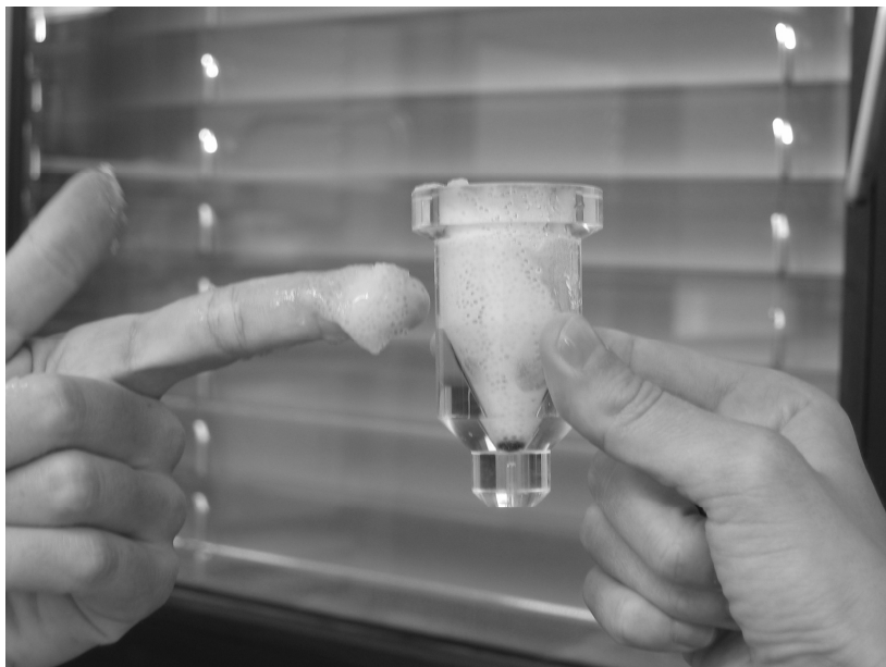
Figure IV.43 Dissolution profile of theophyllin containing Na-CMC micropellets using APP.4 at a flow rate of 10g/min. A blocked dissolution vessel of the APP.4 is observed by a loading of 2g micropellets together with 15g of glass beads (flow rate 10ml/min), described as D7 (n=5).
