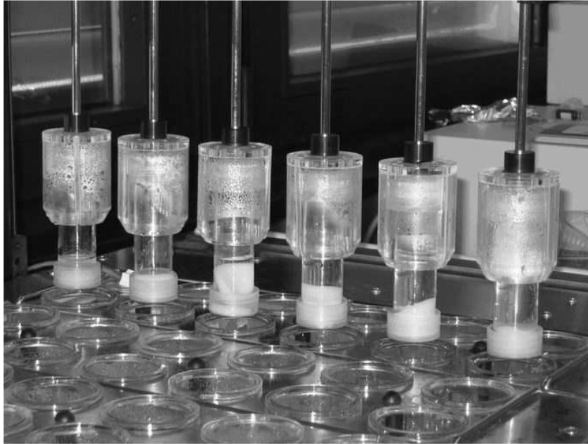
Figure IV.42 Dissolution of theophyllin containing Na-CMC micropellets in the reciprocating cylinder apparatus. The cylinders are still filled with buffer after the drip off time, because they are blocked by the mucoadhesive micropellets.
