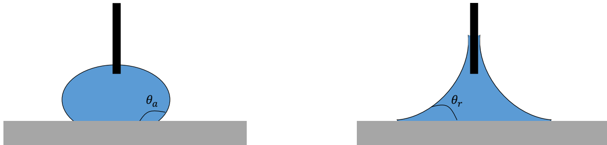
Figure 1.4: Left: a syringe dispenses continuously liquid on a solid surface until the growing drop reaches a constant advancing contact angle \Theta_a . Right: The syringe withdraw liquid, which decreases the contact angle until a constant value called receding contact angle \Theta_r .
