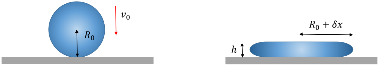
Figure 1.7: Left: Falling drop hitting the surface before starting its deformation. Right: Deformation of the drop upon impact in form of a pancake. The lateral deformation is denoted by \delta x and the thickness of the film as h .
