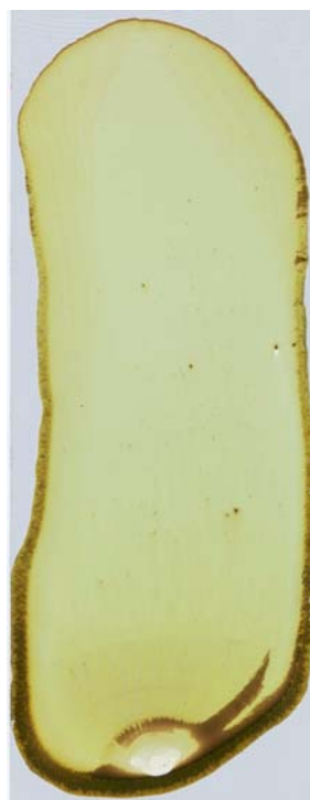
Figure 2.9. Pictures of the PMMA crystalline films prepared on a glass substrate: a) PMMA opals with 367 nm diameter spheres, b) PMMA opals with 275 nm diameter spheres (Sample No. 3), c) same sample as a).
