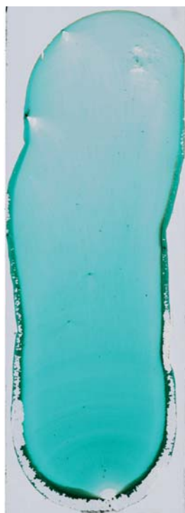
Figure 2.9. Pictures of the PMMA crystalline films prepared on a glass substrate: a) PMMA opals with 367 nm diameter spheres, b) PMMA opals with 275 nm diameter spheres (Sample No. 3), c) same sample as a).
