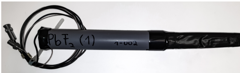
Figure 5.15.: Ready-to-use single crystal calorimeter prototype detector.
