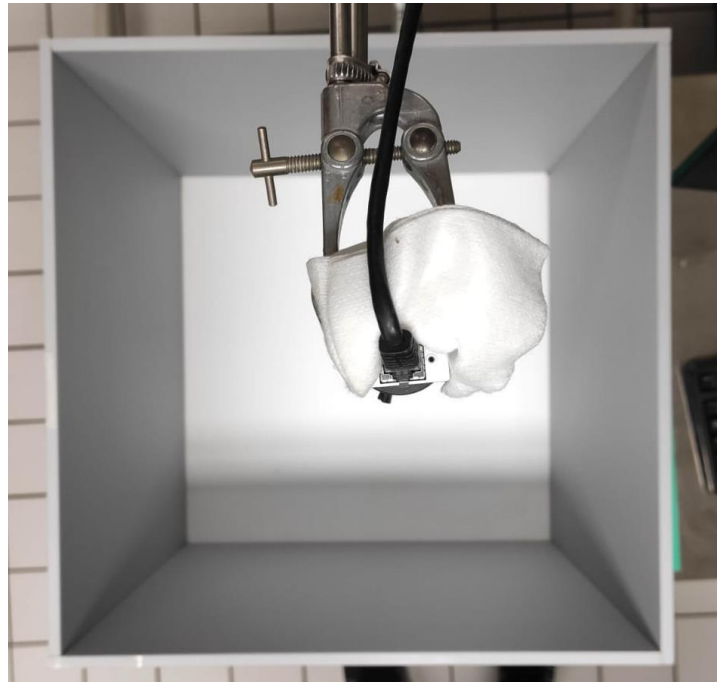
Fig. 9 Ethovision XT Open field test setup for behavioral investigation. The Noldus Ethovision XT setup was used to perform behavioral analysis on transgenic mice. The cubes dimensions are 40x40x40 cm. The high-definition camera observes the field area and tracks the mice from above.
