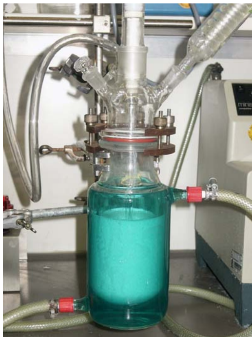
Fig. 2.1: Typical reactor used in the lab for the preparation of polymer latex
