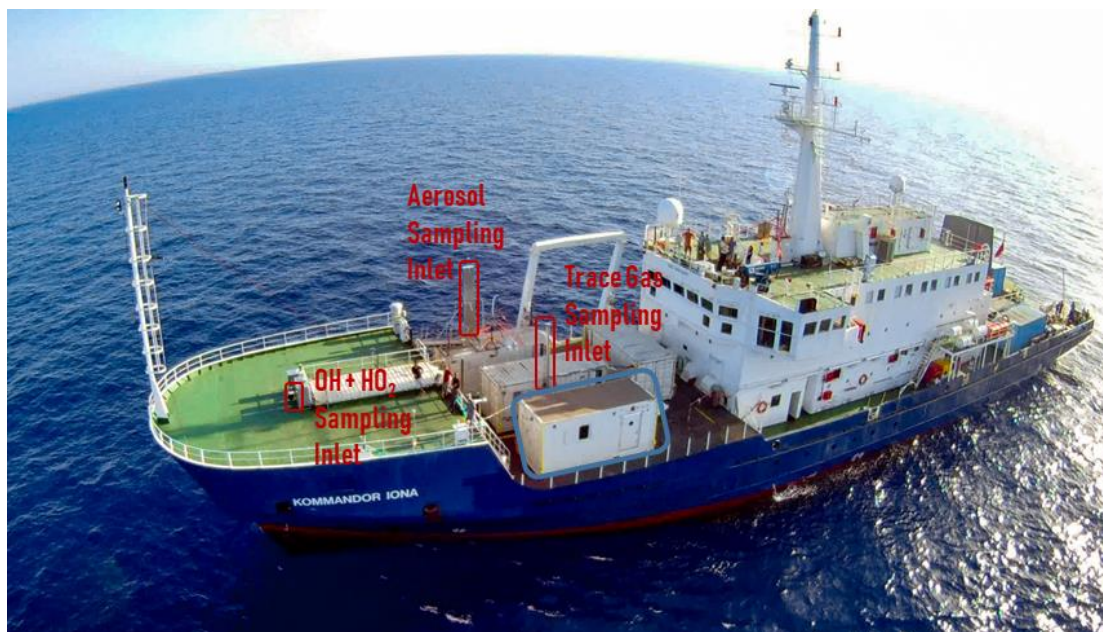
Figure 26: Instrumental setup on the Kommandor Iona . The HCHO, H 2 O 2 , ROOH, CO and NO x instruments were set up in the highlighted lab container and connected to the trace gas sampling inlet via bypass tubing with high flow rates. The HO x and aerosol instruments had separated sampling inlets, specialized with regards to the needs of the respective instrumentation.
