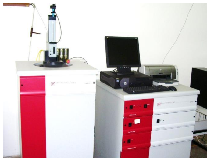
Figure 3.1. The experimental setup of SQUID magnetometer used in the present research.
