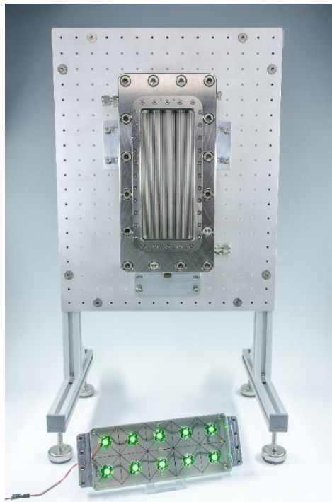
Figure 14: FFMR-LARGE for photochemical applications mounted on a rack (©Fraunhofer IMM).
