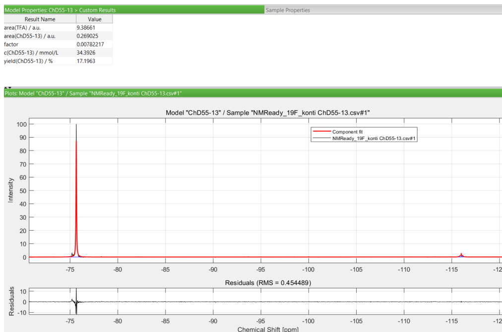
Figure 265: Evaluation of an online 19 F-NMR spectrum (56.98 MHz, PEEK flow cell) with PEAXACT 5.3 (component fit via IHM) of continuous 31b synthesis in a 1/16" FEP capillary photoreactor; General reaction conditions: 200 mM 4-fluoroaniline, 1.2 equiv. t -BuONO, 2 equiv. TFA in MeCN, MeCN/benzene V/V=1/1, 365 nm 50 W el , 20 °C, 17 bar exs , t R =1.25 h; blue peak shape of each pure component fits (and unknown substances), red component fit as result of a weighted sum of pure components; top: Results of component fitting including yield of continuous 31b synthesis.
