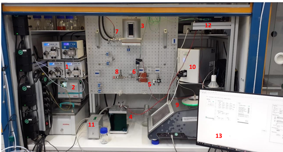
Figure 67: Complete lab plant including a reactors, online spectroscopy tools and control unit: 1 HPLC-pumps, 2 thermostat, 3 1/8" thermal reactor, 4 1/16" capillary photoreactor, 5 liquid-liquid separator-Zaiput Sep-10, 6 pressure sensor, 7 external thermocouple of thermostat T_{\text{ext}} , 8 back pressure regulator (spring loaded), 9 benchtop-NMR-spectrometer, 10 ATR-FTIR-spectrometer, 11 IR-sensor, 12 interphase, 13 control unit + software (computer).
