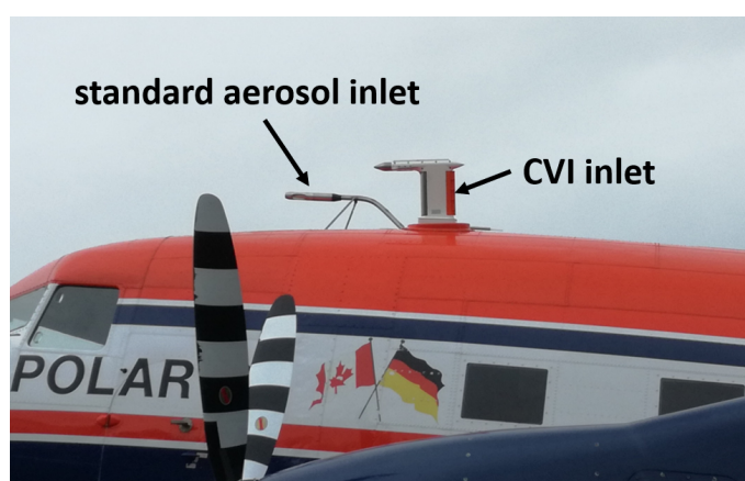
Figure 2.7: Picture of both aerosol inlets (standard aerosol inlet and CVI) mounted on top of the Polar 6 .
