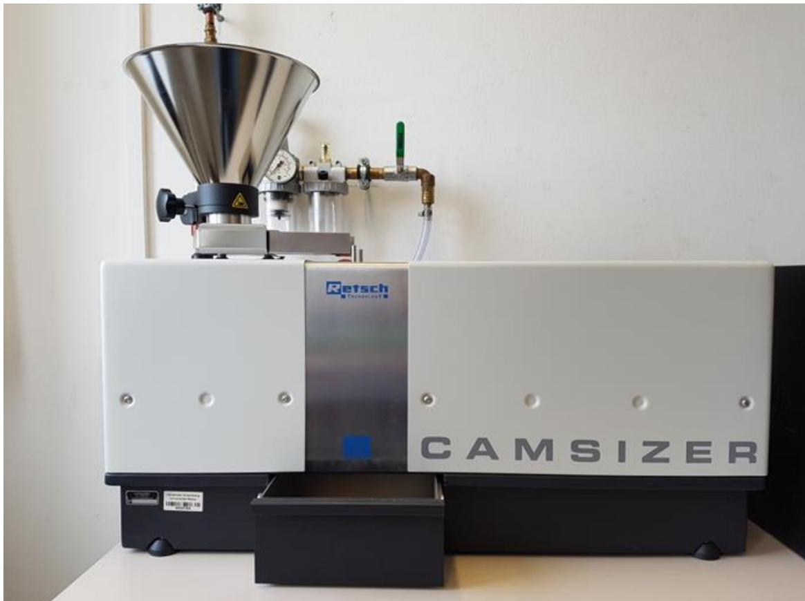
Fig. 3.1: Camsizer ® device with sediment funnel and feeding channel on top left.
