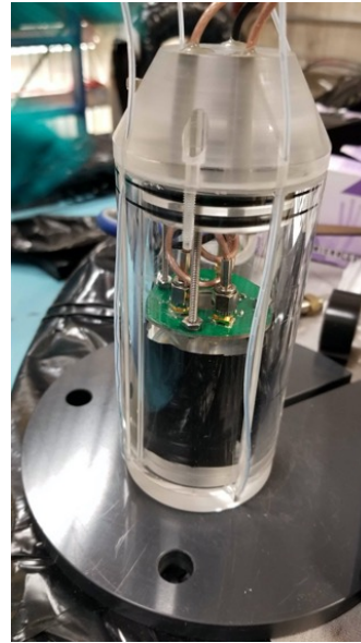
Figure 5.33: Left: Schematic cross-section view of the AmBe source. Detection of scintillation light emitted by the gamma in the BGO with the SiPMs provides the tag for the neutron emission. Figure based on [225]. Right: Picture of the AmBe source in the housing.
